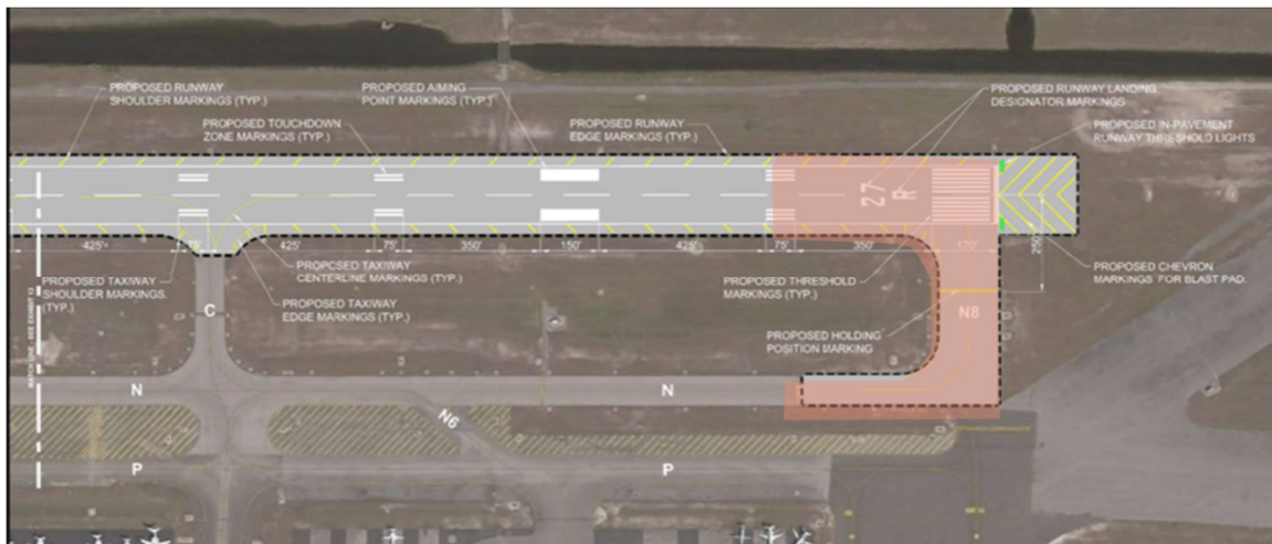
Figure 3-3 - RW 27R (east end) – Full-Depth Reconstruction
