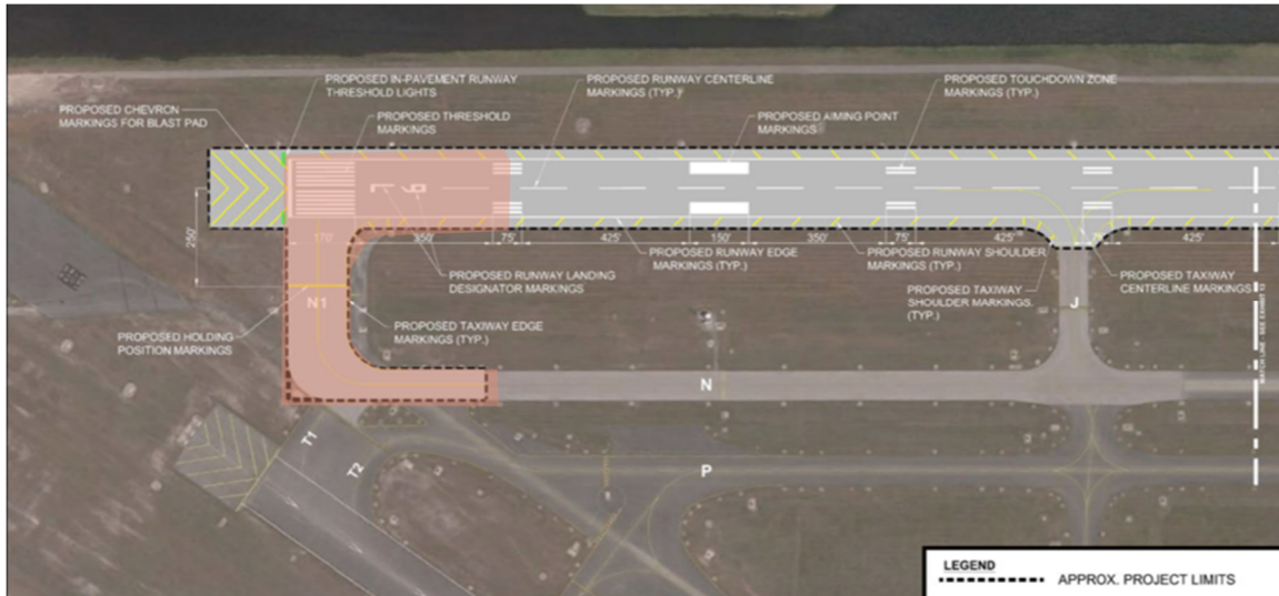
Figure 3-1 - RW 9L (west end) – Full-Depth Reconstruction
